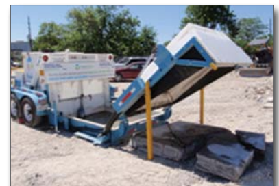
Figure 17. Delivering hardened concrete to a recycler
